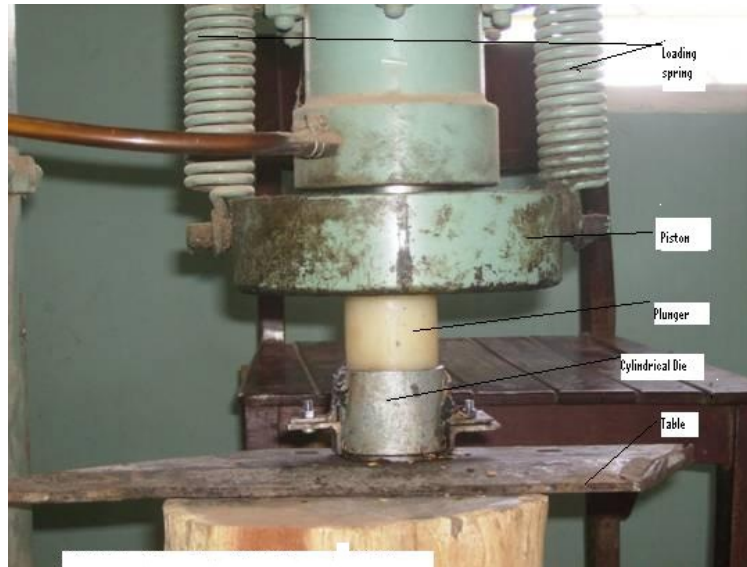
Figure 1. Hydraulic powered press fitted with plunger and cylinder die.
